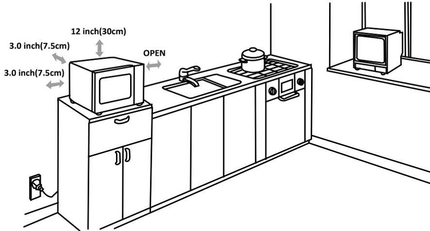
The rear surface of appliance shall be placed against a wall. A minimum clearance of 7,5 cm is required between the oven and any adjacent walls. One side must be open.
