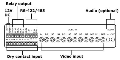
The back panel of the 12-audio-input version consists of:
