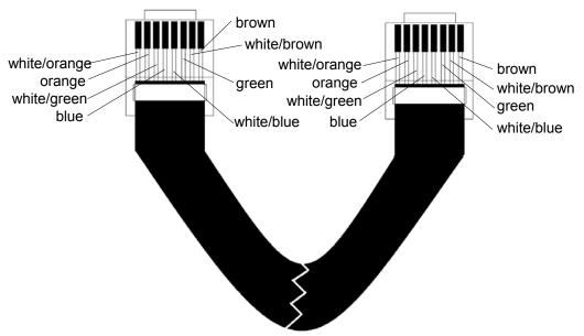
Here is the bottom view of the RJ-45 connectors on a crossover cable:
